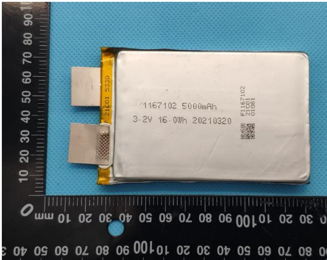
Cells /电芯 (1167102 3.2V 5000mAh 16Wh)
